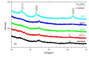
**Figure 1**: XRD patterns of: (a)  $Fe/SiO_2$ , (b)  $Fe-Ni/SiO_2$  and (c)  $Fe-Co/SiO_2$ .
