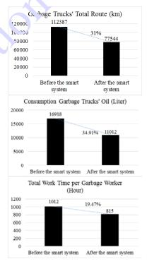
Figure 9. Smart waste collection efficiency.
