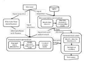
Figure 3. Detailed design of test case generation.
