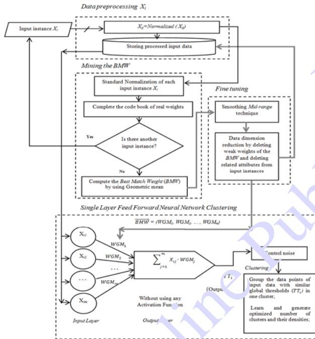
Figure 1. The design of the RUFFNN clustering method.
