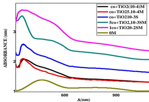
Figure 2: UV–visible absorbance spectra of (P3T+6T)/ITO and ((P3T++6T)+TiO<sub>2</sub>)/ITO films, obtained for various contents of TiO<sub>2</sub> (0, 10<sup>-4</sup>, 5.10<sup>-4</sup>, 5.10<sup>-3</sup>, 10<sup>-3</sup> and 10<sup>-2</sup> M).
