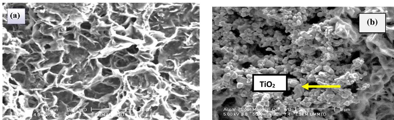
**Figure 3:** Micrographs of unmodified P3T+6T/ITO (a), and (P3T+6T+TiO<sub>2</sub>)/ITO (b) films
