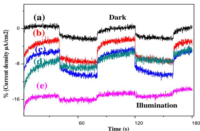
**Figure 5:** Current density-time plots of P3T+6T/ITO and (P3T+6T+TiO<sub>2</sub>)/ITO films with different concentrations of TiO<sub>2</sub> (C = 0, 10<sup>-4</sup>, 5.10<sup>-4</sup>, 10<sup>-3</sup>, 5.10<sup>-3</sup> and 10<sup>-2</sup> M), in CH<sub>2</sub>Cl<sub>2</sub>/TBAP (0.1 M) at a potential of -400 mV, observed on switching the light on and off for 100 mW.cm<sup>-2</sup> light intensity.
