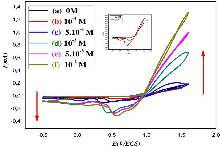
**Figure 1** : Cyclic voltammograms during the polymerization of a composite film in  $\text{CH}_2\text{Cl}_2/\text{TBAP}$  ( $10^{-1}$  M) aqueous solution obtained for different concentrations of  $\text{TiO}_2$  ( $C = 0, 10^{-4}, 5 \cdot 10^{-4}, 10^{-3}, 5 \cdot 10^{-3}$  and  $10^{-2}$  M), obtained with scan rate of 10 mV/s, over a potential range of -0.3 to 1.6 V/SCE by using a Pt electrode ( $\varnothing = 2$  mm).
