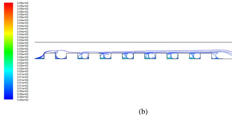
FIGURE 4. The isotherm lines of the turbulent flow around the ribs at  $Re= 9.4 \times 10^4$ :
